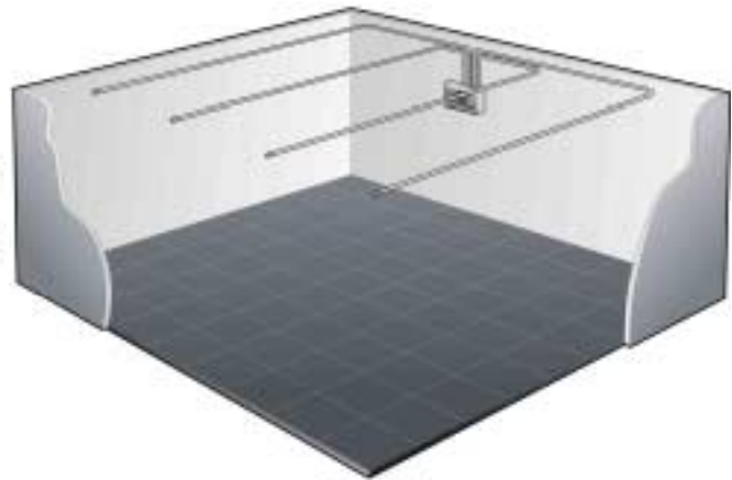
Figure 2 - Standard room sampling layout
