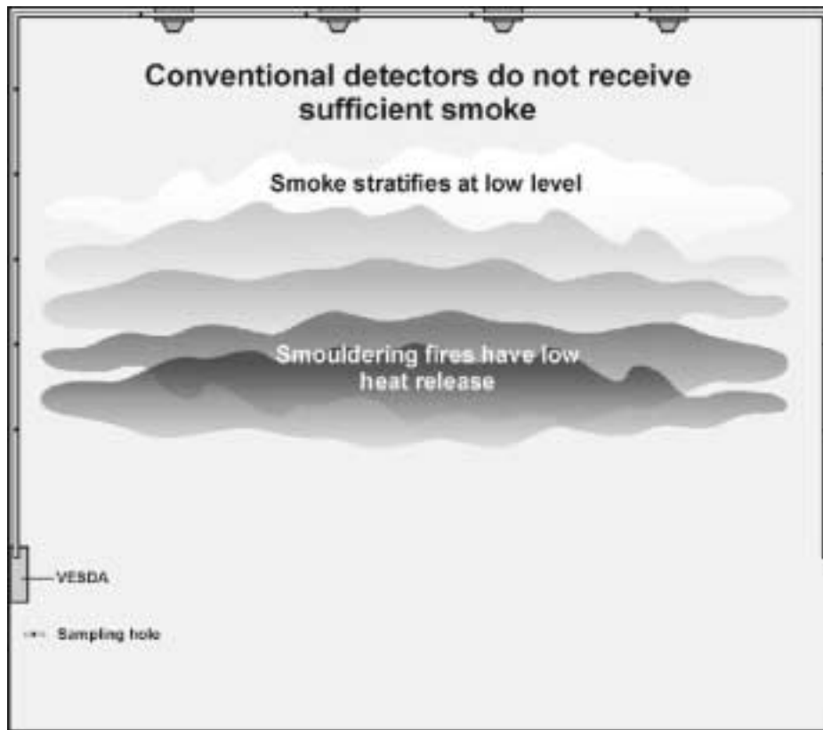
Figure 5 – Smoke stratification: VESDA multiple level sampling v's conventional detectors.
