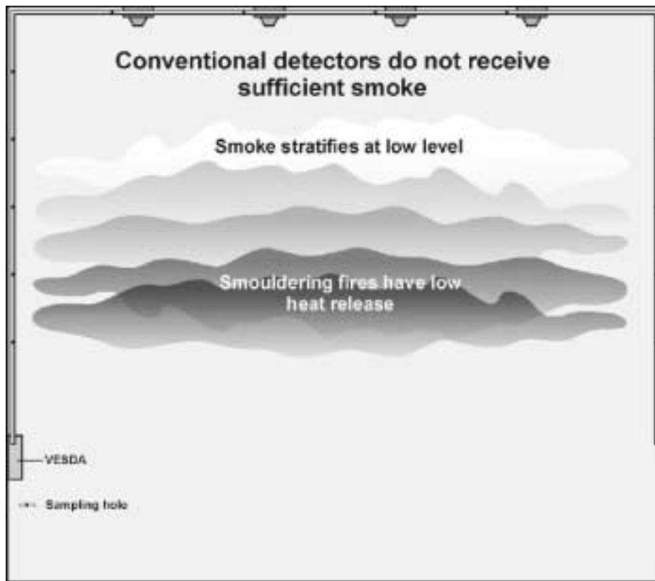
Figure 4 – Smoke stratification: VESDA multiple level sampling v's conventional detectors.
